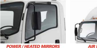
Heated flat and convex mirrors with or without dual remote controls. Heated mirrors prevent fogging and ice collection with a quick push of a cab switch. For added convenience, available remote controls allow the driver to quickly adjust the angle of the mirrors.
