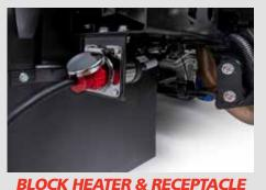
Warms engine coolant for more efficient cold engine start up. Reduces the need for prolonged engine warm-up.
