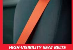
High-visibility orange seatbelts provide quick visual verification that seat belts are being worn to conform with safety regulations. (Driver and right passenger seat only.)
